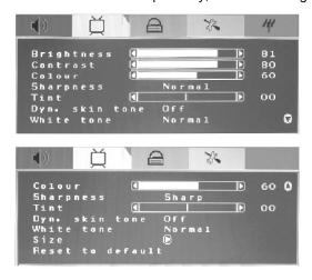
When the input source is in **Component** mode, you can select Brightness, Contrast, Colour, Sharpness, Tint, White tone, Size and Reset to default respectively; shown in the figure below:
